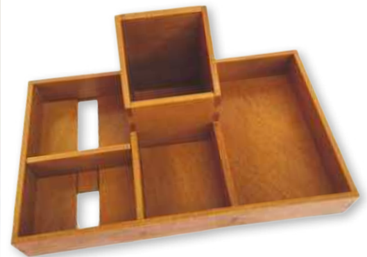
▲ Pic.17 The completed desk-tidy after sanding and a coat of lacquer spray
